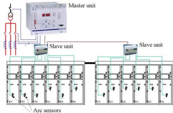
FIGURE 4: Structure of an arc protection system.
