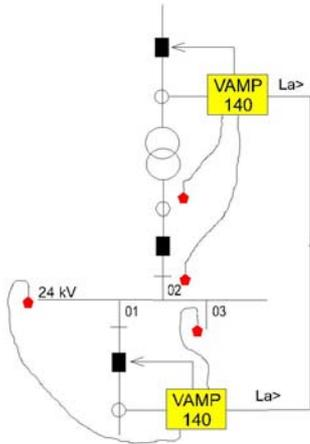
**FIGURE 7: Arc protection system using overcurrent relays with arc sensor option. Information about the activation of the arc sensors may be carried between the relays using the binary inputs and outputs (La>).**
