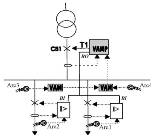
**FIGURE 6: Overcurrent relays with arc sensor option and specialised arc protection system (VAMP and VAM). Information about activation of arc sensors Arc3 and Arc4 is also brought to the overcurrent relays via the binary inputs (BI).**
